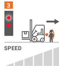
When the sensor, placed on the rear part of the vehicle, detects an obstacle **Safe&Stop**, immediately alert the operator through visual and acoustic alerts. In addition the system can intervene on the speed of the vehicle (\*) in two steps strongly reducing the risk of collision and accident.
