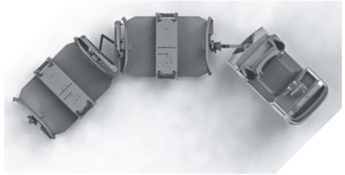
The folding tiller enables drivers to manoeuvre through corners and shelving aisles with flexibility
