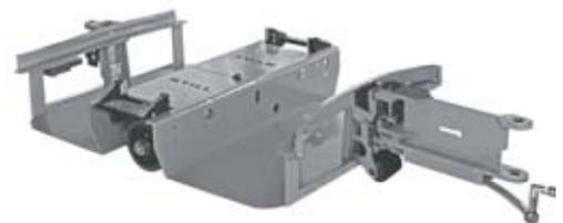
LiftRunner B-Frames are designed for different types of trolleys up to 1,000 kg. They offer maximum flexibility on different routes thanks to the option of loading and unloading from both sides without decoupling the frame. To guarantee their directional stability even at higher speeds and during braking manoeuvres the two-wheeled frames are steered via a centre axle. The combination of rigid and flexible links keeps the entire train stable in all driving situations and also
