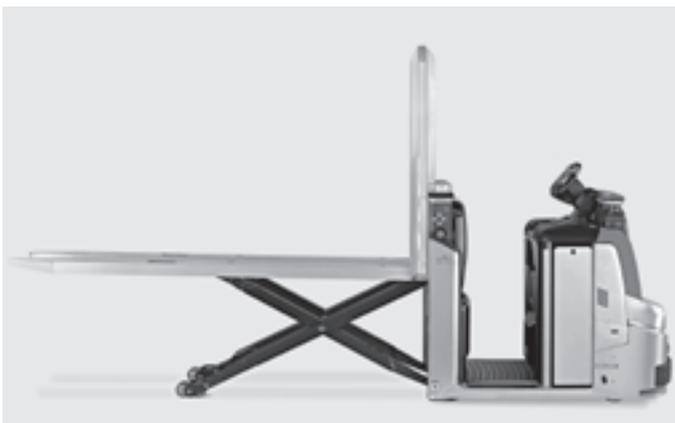
The right level: freely adjustable lifting heights on the OPX-L 20 S iGo neo variant for additional ergonomics
