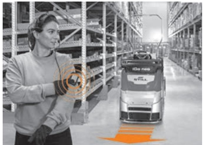
Process reliability – even for empty racks or crossroads: the OPX iGo neo recognises and passes by empty racks. Crossroads are also detected well in advance and the truck will only drive autonomously over them once the driver has checked the way is clear and has approved the onward journey.
