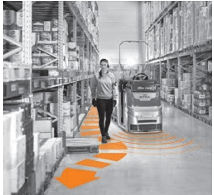
Precise handling in the event of obstacles: the OPX iGo neo autonomously avoids obstacles and reacts to the situation. Trucks will either drive around the obstacle, avoid it by driving in convoy, or – if the obstacle completely blocks its path – the truck will stop.
