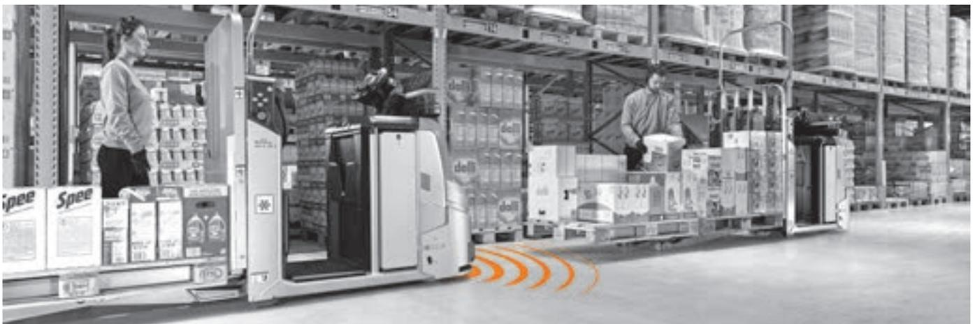
Speed is adjusted to the surroundings: if a slower truck is moving in front, or if a queue forms, the OPX iGo neo will intelligently adjust its speed to the situation. If the operator decides to travel on foot while the truck waits in the queue, then the truck will autonomously start driving again once the queue has resolved itself.
