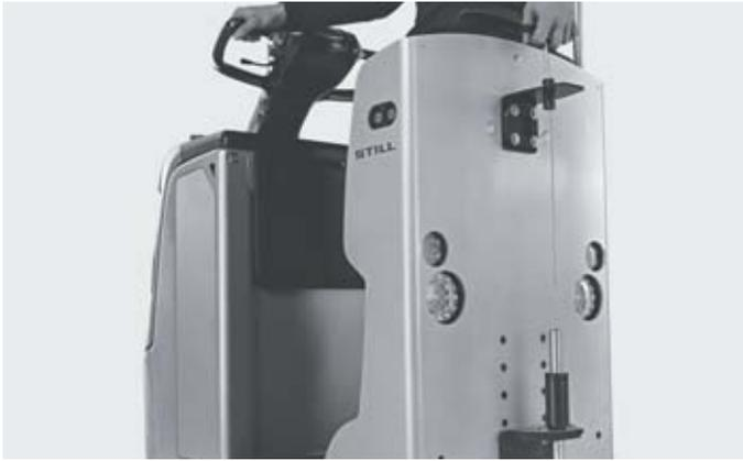
Fast release of coupling from driver's seat<sup>1</sup>
