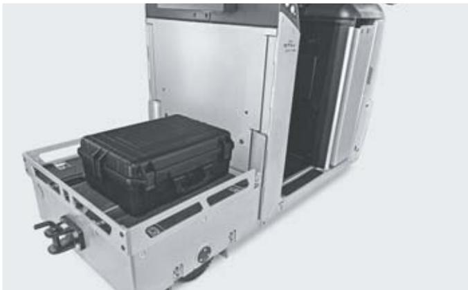
Storage surface with lashing eyelets for up to 600 kg<sup>3</sup>
