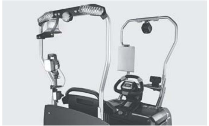
Optional accessory bar for versatile application options and many equipment options including flash lights and working lights<sup>2</sup>
