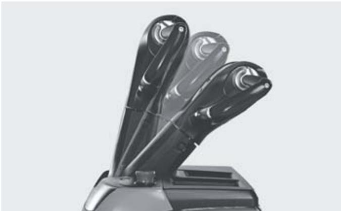
Height-adjustable steering for different drivers<sup>1</sup>
