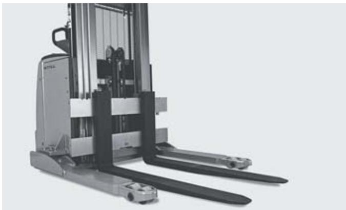
All-rounder: self-supporting and adjustable forks allow the handling of different pallet types <sup>1,2</sup>
