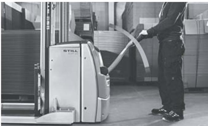
Safety as standard: depending on tiller angle, speed is automatically adapted to the distance between the operator and the truck (OptiSpeed) <sup>1,2</sup>
