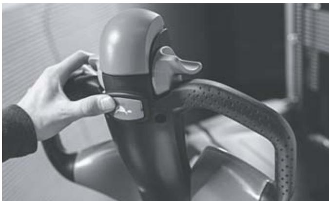
Precise in any situation: thanks to creep speed it is possible to manoeuvre in the most confined of spaces <sup>1,2</sup>
