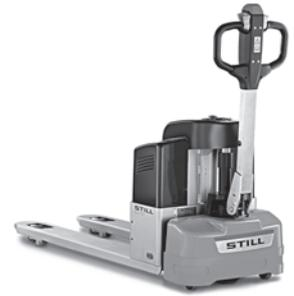
Be it in industrial applications, retail or logistics – with the ECU 15 C, STILL offers more than just one good reason to dismiss hand pallet trucks into retirement. The low lift pallet truck scores with a range of quality aspects: driving, lifting and lowering – all this is done electrically and without any physical force by the operator.
